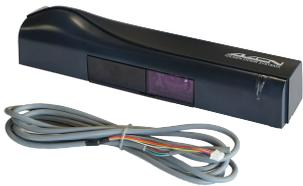
Motion detector: Zur Montage am Türkasten vorbereitet, detection method: Bewegung, detection fields of radar are adjustable, wide field 4 m (W) x 2 m (D), narrow field 2 m (W) x 2,5 m (D), supply voltage 12 ... 24 VAC or 12 ... 30 VDC, power supply via connector on door plate.
