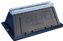
The nVent CADDY Pyramid ST Fixed Strut Support offers a simple and adaptable solution for mounting electrical and mechanical services on commercial rooftops. This support system is engineered to evenly distribute weight across the base, ensuring optimal load management. Additionally, the foam pad on the underside provides a low-abrasion interface that protects roof membranes, eliminating the need for a slip sheet.
