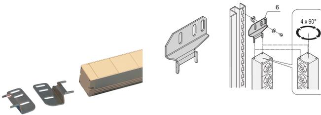
Assembly kits for PDUs. Allows easy integration of PDUs in a rack.
