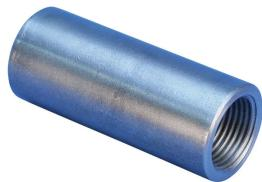
Stainless steel couplers are specified whenever corrosive environmental conditions combine with the need for high load-bearing strength. nVent LENTON stainless steel couplers are commonly used when the construction materials may come into contact with de-icing salts, salt water or marine environments. Typical applications include bridges and bridge decks.
