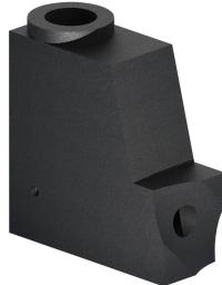
Side fill angular pouring basins are used when interferences of the structure will not allow top filling of the sleeve and the interferences are directly next to the tap hole in the sleeve.
