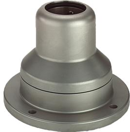
CS480 Swivel Base External allows the entire suspension system to rotate at the point of attachment on a horizontal surface. Arm can be rotated or turned 340 degrees. Base mounting hardware is exposed. Maintenance-free bearings.
