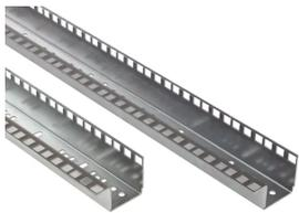
19-in. Rack Angles are available in square-hole and tapped-hole designs. Tapped Rack Angles are 12 gauge plated steel with 10-32 tapped holes. Square-Hole Rack Angles are 14 gauge plated steel designed to accept metric or English cage nuts. 19-in. Rack Angles are fixed directly into a 600-mm wide enclosure frame. To mount 19-in. Rack Angles in 700- or 800-mm wide frames, use frame reducing brackets.
