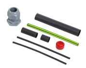
nVent RAYCHEM CE20-01, CE20-03 and CE25-01 are heat shrink polymer kits used to connect and terminate select nVent RAYCHEM self-regulating trace heating cable. Requires wire stripping and a heat gun. Each kit contains connection components for a cable termination and end seal.
