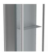
This polycarbonate horizontal separation plate, MSIS, is available off the shelf and pre-sized. The plate should be used when subsections need to be segregated. It is placed between a mounting plate and a front panel that is placed inside the enclosure. No screws are needed, which makes mounting easy. The fix section can then comply to up to form 4 segregation according to IEC 61439.
