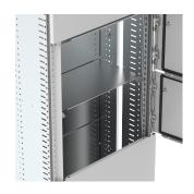
This polycarbonate horizontal separation plate, MSES, is available off the shelf and pre-sized. The plate should be used when subsections need to be segregated. It is placed between a mounting plate and the doorway for partial doors. No screws are needed, which makes mounting easy. The fix section can then comply to up to form 4 segregation according to IEC 61439.
